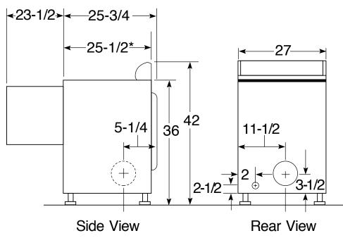
\*24-1/2" from the edge of the side panel to the front. 25-1/2" from front to edge of end caps.
